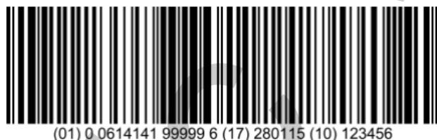
Figure 3-10 A GS1-128 Barcode Encoding a GTIN, Expiration Date and Batch/Lot
